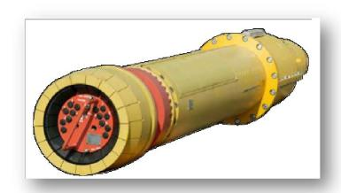
as a result of deep water depths. Collet connectors consist of collet-style "finger" design which firmly locks around a mating hub. Collet connectors are used for both vertical and horizontal jumper spool connections and are available in both integral hydraulic and mechanical (with separate actuation tool) configurations. Clamp connectors consist of a two piece segmented clamp design and are particularly well suited for
