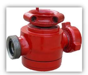
We provide ULT and DR Plug valve which are our premium, quarter-turn valve designed for a wide range of standard and sour gas drilling, production and well-servicing applications. These valves are offered in single and dual body design in pressures to 20,000 psi. They range in size from 1 to 4 inches and come with threaded unions, flanged and clamp hub ends
