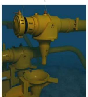
umbilicals and Jumper spools. The termination head is hauled in to the Tie-in point by use of a subsea winch. Horizontal Tie-in may be made up by Clamp Connectors operated from a Tie-in tool, by integrated hydraulic connectors operated through the ROV, or by non-hydraulic collet connectors with assistance from a Connector Actuation Tool (CAT) and ROV. Horizontal connections leave the flowline/umbilical in a straight line, and is easy to protect if overtrawling from fishermen should occur.
